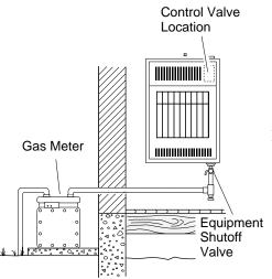
Figure 14 - Checking Gas Joints
